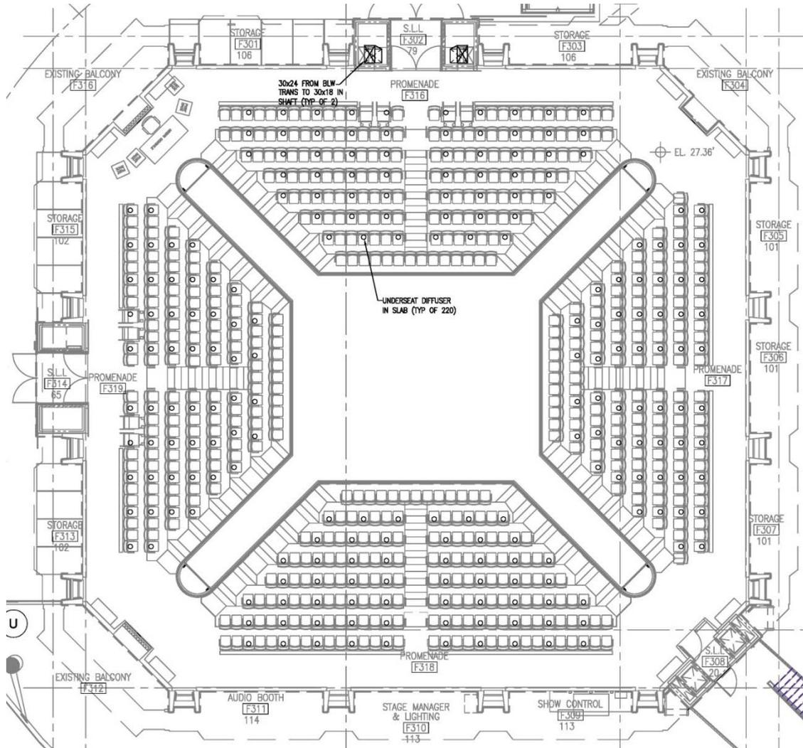
**Figure 13: Mechanical Plan MH-132 (Level 27.5') – Underseat Diffusers**
