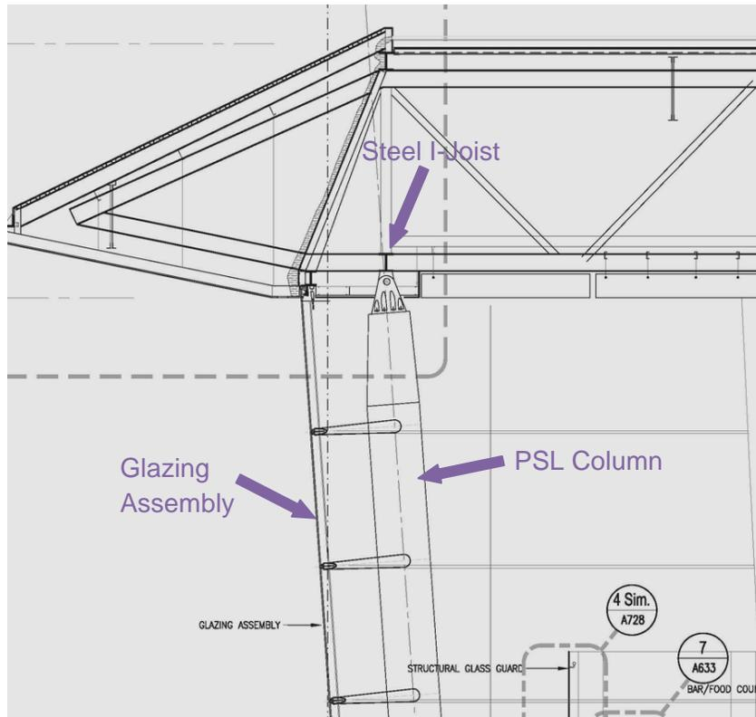
**Figure 3:** Wood, glass, and steel connection at the curtain wall
