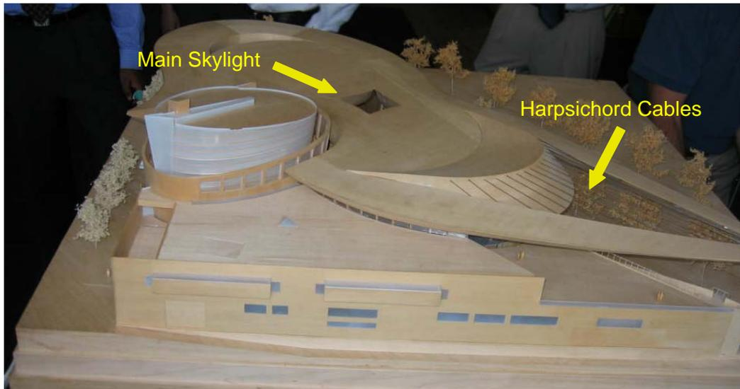
**Figure 9:** The old model showing the “harpichord” cantilever support and the main lobby skylight
