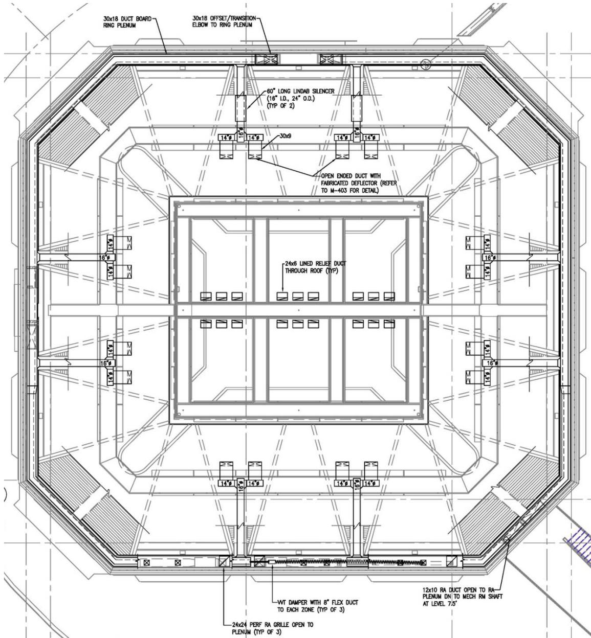
Figure 12: Mechanical Plan MH-142 (Level 43.0') – Ring Plenum
